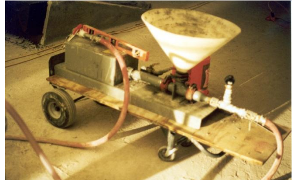
Figure 4.2 - Vacuum Grouting Equipment, Digital Volumeter (up (upper left), Void Volume Measurement (upper right), Grout Pump (lower left), Vacuum Grout injection (lower right)
